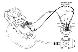
With a built-in hand pump, precision measurement of both pressure and current, the Fluke 718Ex Pressure Calibrator is a complete, self-contained tool for the calibration of P/I transmitters. To calibrate a 3 psi to 15 psi/4 mA to 20 mA transmitter using a Fluke 718Ex 30G Pressure Calibrator:
