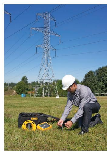
For the 3-pole Fall-of-Potential test, two earth stakes are placed in the soil in a direct line—away from the earth electrode.
