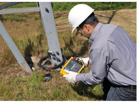
Stakeless measurement is possible by measuring earth ground loop resistances for multi-grounded systems using only current clamps. This test technique eliminates the dangerous and time-consuming activity of disconnecting parallel grounds, as well as finding suitable locations for auxiliary ground stakes. You can also perform earth ground tests in places you might not have considered before: inside buildings, on power pylons, or anywhere you don't have access to soil.
