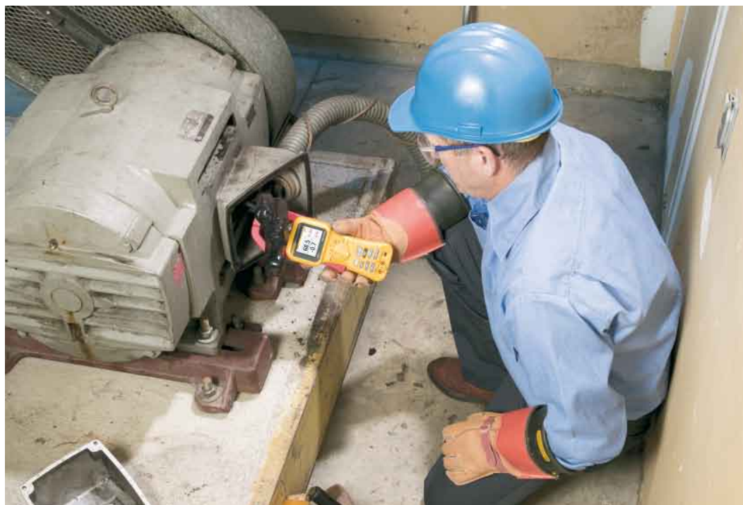
Figure 1. The dual waveform display on the Fluke 345 shows both voltage and current waveforms.
