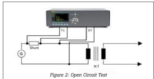
Figure 2: Open Circuit Test
