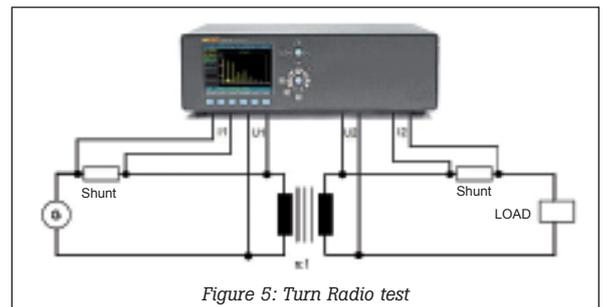
Figure 5: Turn Ratio test
