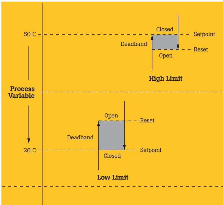
Figure 1. 2-point switch with settings for low and high setpoints.
