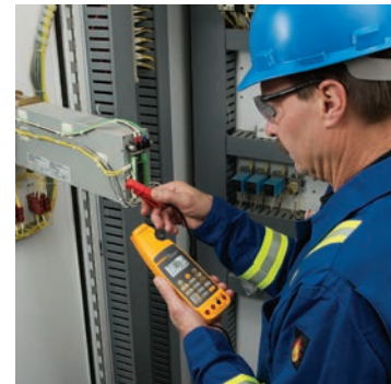
Measure process and other automation 4 to 20 mA signals without breaking the loop.
