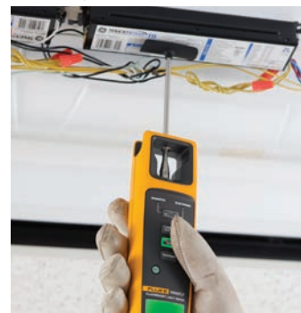
Easily determine if ballast is working.
