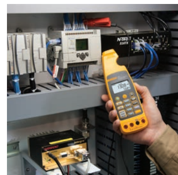
Measure process and other automation 4 to 20 mA signals without breaking the loop.
