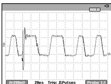
**Figure 3.** Broadcast signal with a voltage spike occurring at the waveform transition, corrupting the intended fieldbus message.
