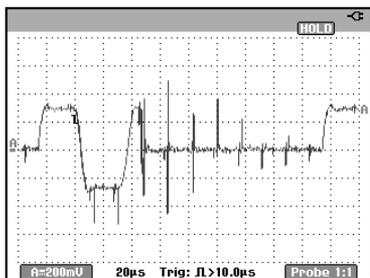
**Figure 2.** Broadcast signal with approximately 1 Volt p-p noise.
