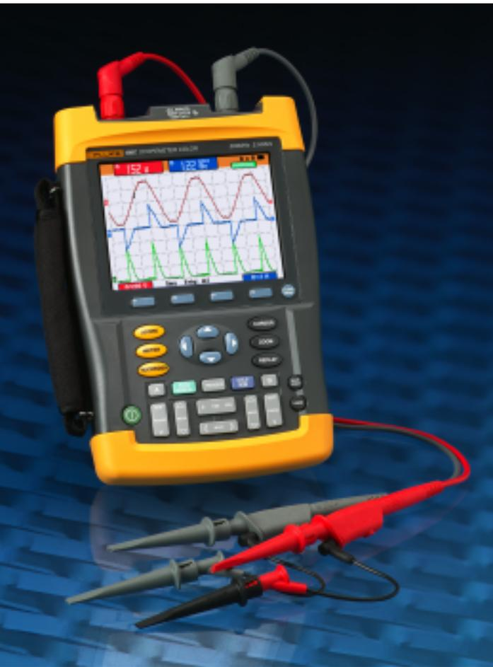
The portability of Fluke's latest color ScopeMeter® test tool and its ability to store screen traces for later downloading to a PC has proved a winner with Balfour Beatty Rail Infrastructure Services. The handheld oscilloscope is proving invaluable in saving time and manpower to troubleshoot trackside electrical problems on a section of the rail network managed from the London Bridge control center. These electrical faults commonly occur throughout much of the aging UK rail network.
