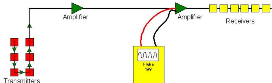
At each interface with the trackside equipment there is a “hand cut read” device and a transmitter which reads or writes signals at the unit’s designated channel frequency. In the past, when a unit failed it typically took an average of 12 hours for a maintenance person to walk the signal line, checking each unit one-by-one until the fault was found. Now a rapid solution to the problem is available using the Fluke ScopeMeter test tool.
