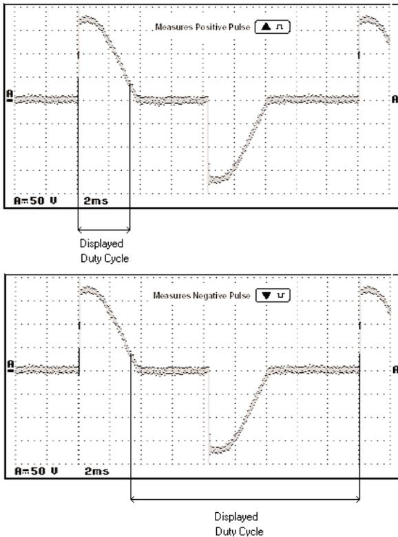
Figure 2. Trigger set for positive pulse
