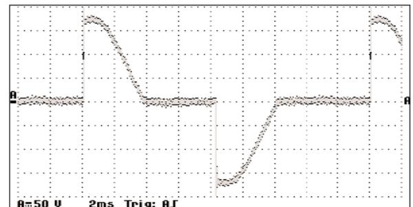
Figure 1. SCR output at approximately 50 percent
