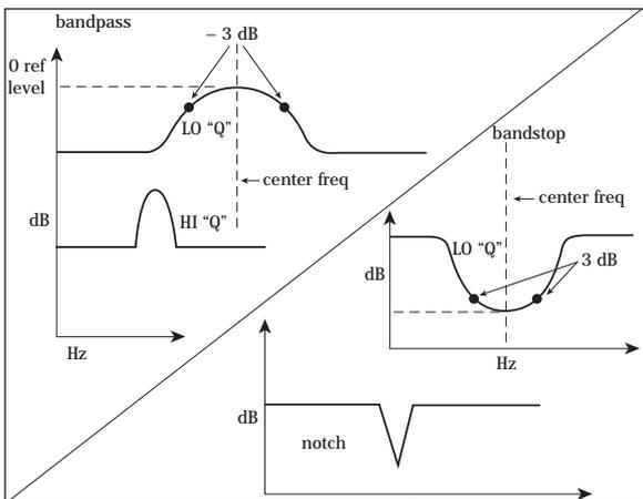
Figure 4. Bandpass and stopband output response plots
