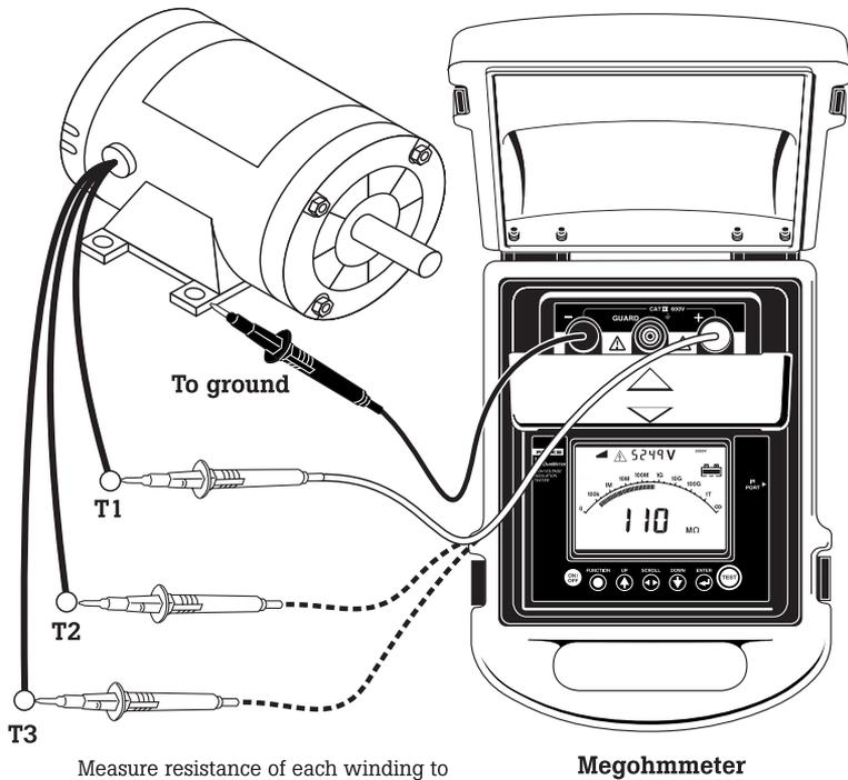
Measure resistance of each winding to ground and record reading on graph.
