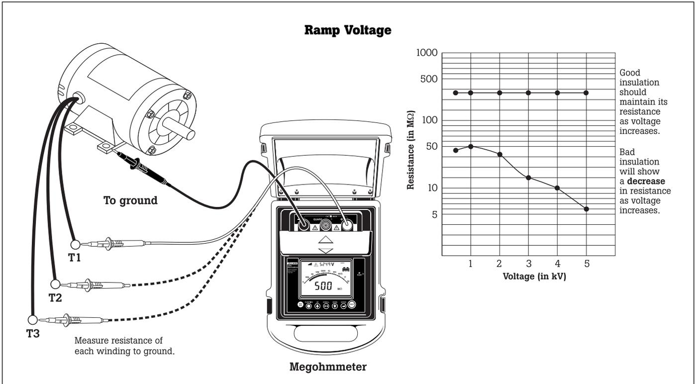
Step voltage or ramp voltage testing can find insulation prone to fail due to arcing.
