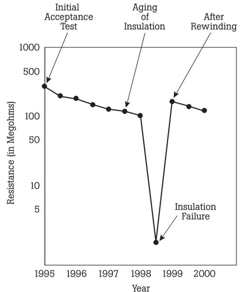
Periodic spot check can be used for preventive maintenance, but must be adjusted for temperature and humidity.
