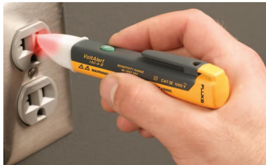
Try this yourself with a pair of two-prong extension cords. Plug one cord into a wall outlet and plug the second cord into the first but connect only the hot side leaving the neutral open. Go to the loose end of the second cord and try the voltage sensor in both sides. They both should indicate live voltage.
