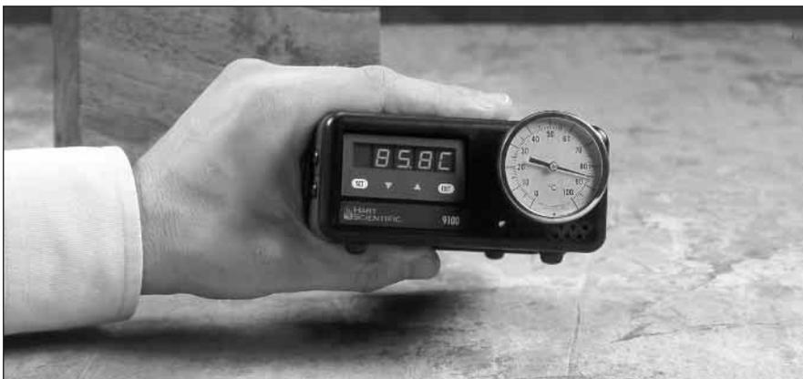
*With developments in dry-well technology, precision temperature calibration can be performed in the field.*
