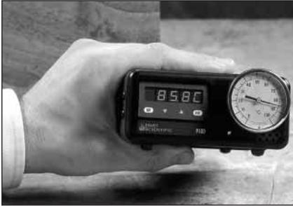
**Handheld block calibrators have made industrial calibration more portable.**
