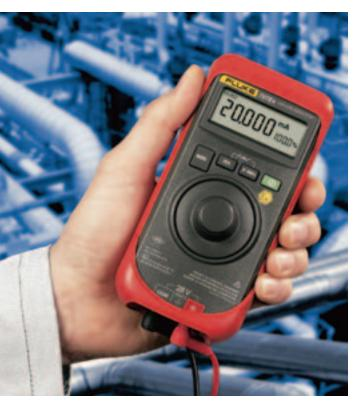
Tracking down problems within a process loop can be a difficult challenge in the best of environments. Doing so in an area that has the potential for explosion takes the degree of difficulty to another level – one where the technician needs proper training and equipment. This article will demonstrate the practical application of loop calibrators designed to troubleshoot process loops in intrinsically safe environments.
