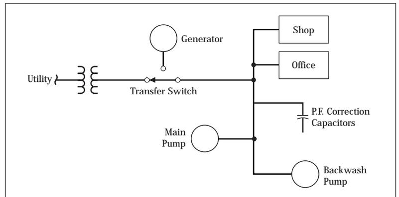
Fig. 1 One-line diagram of the water plant
