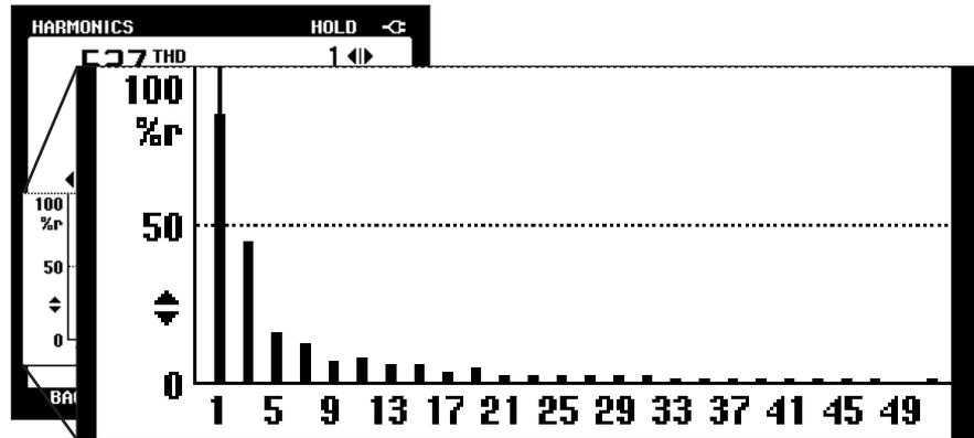
Fig. 2 Example of a normal ac current spectrum with all odd harmonics
