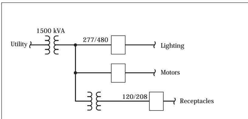
Fig. 1 Partial one-line diagram of large commercial building
