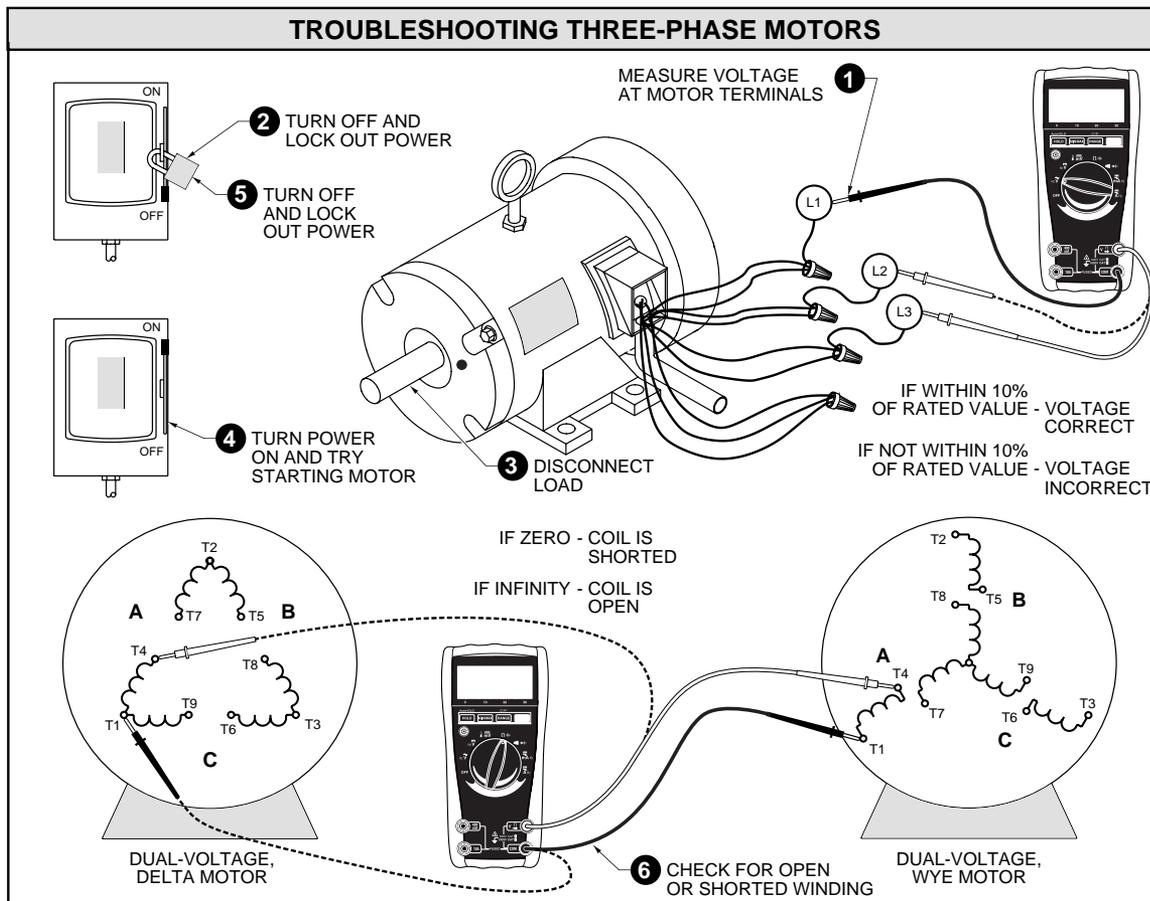
Figure 1. Troubleshoot three-phase motors with an ohmmeter.
