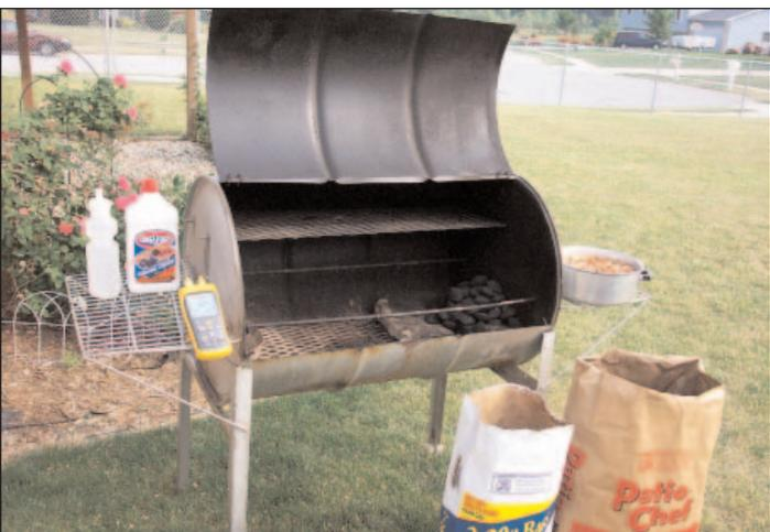
Afterwards, Huerta can download the data to a PC and, using FlukeView Forms software, chart the temperature of both channels over time. (See accompanying charts). The charts show sharp drops in temperature inside the barbecue that coincide with Huerta opening the lid to add wood chips or slather sauce on the meat.
