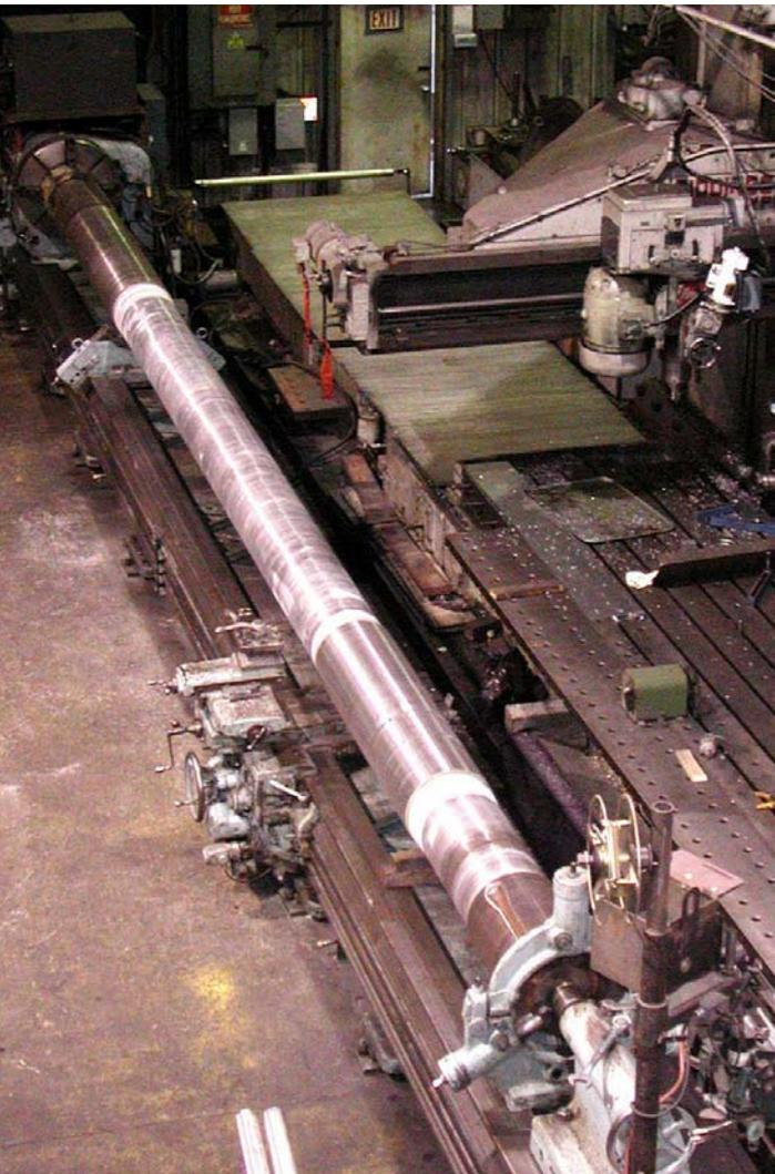
A large propeller shaft before a stress relief and after a weld repair.
