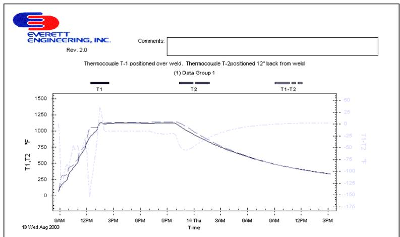
anywhere from 30 seconds to 2 minutes to download the data onto the PC.
