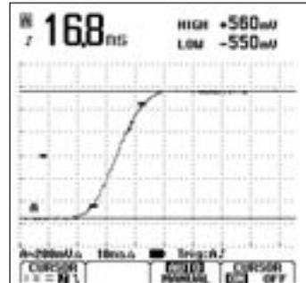
**Figure 5:** Fluke 124 measuring rise time automatically
