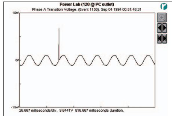
Figure 1 illustrates a peak detect impulse capture. When set at a sampling rate of 8 kHz, which permits capture of transients and impulses down to 130-msec duration, it is adequate for capturing power factor capacitor switching transients but not fast enough for recording high-speed impulses that occur inside facilities due to loads (motors, etc.) turning on and off.
