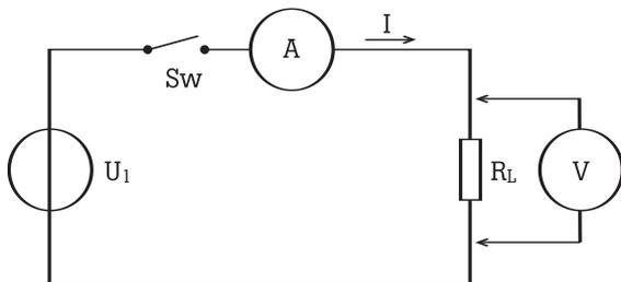
Figure 1. Basic circuit loop in which voltage and current are measured.
