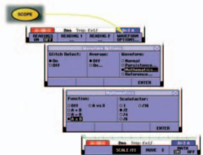
Figure 3. Menu tree for setting up the waveform multiplication.
