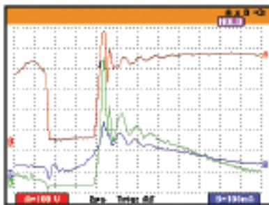
Figure 7. Voltage and current waveforms are used to create the power-curve.
