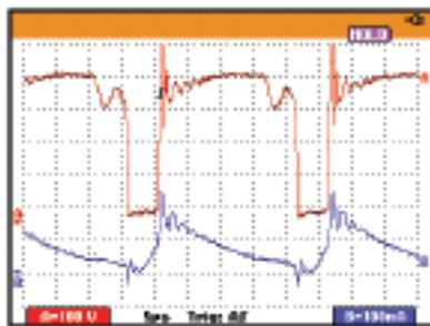
Figure 6. Voltage and current handled by the switcher component in a SMPS.
