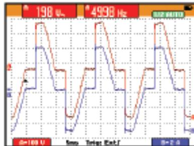
Figure 2. Output voltage and current of a dimmer driving a string of lights.
