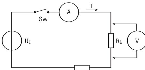
Figure 10. Adding a current sensing resistor to the circuitry to allow current measurement.
