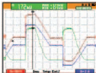
Figure 5. The ScopeMeter's cursor is used for power measurement at a specific point in time.
