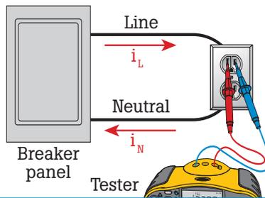
Loop impedance is another another way of thinking about voltage drop. The loop being tested starts at the panel, passes through the tester, and returns to the panel. High loop impedance is a strong indicator of a problem; bad connections, or too long a run for the wire diameter.
