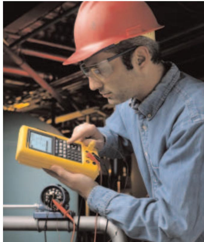
The Fluke 744 HART documenting process calibrator allows technicians to calibrate, maintain, and document HART-based field devices without the need for additional equipment.
