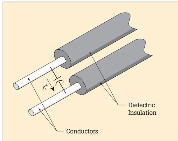
Figure 3. Capacitive charging leakage current ( $I_C$ )
