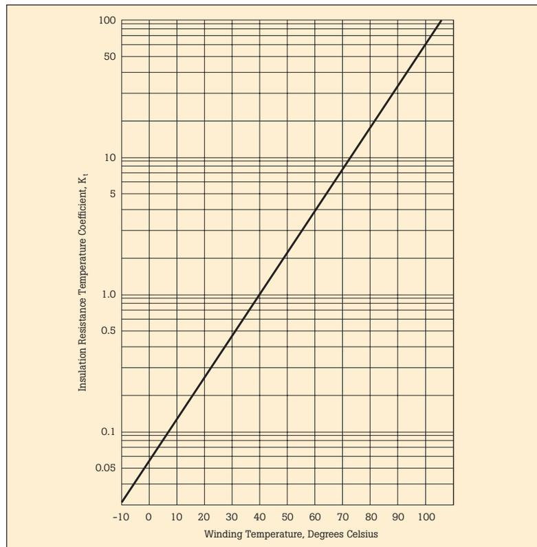
Figure 10. Approximate temperature coefficient for rotating machines
