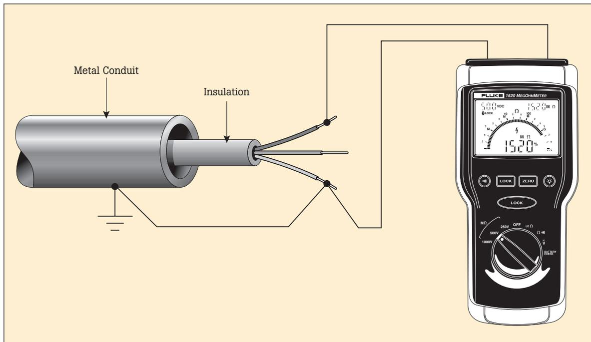
Figure 4. Conductor under test
