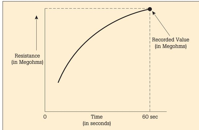
Figure 5. Insulation resistance test
