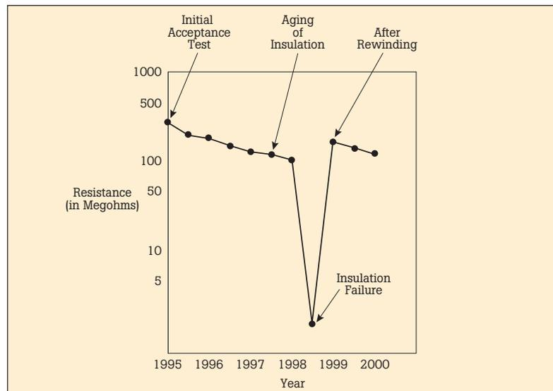
Figure 6. Insulation resistance over a period of time
