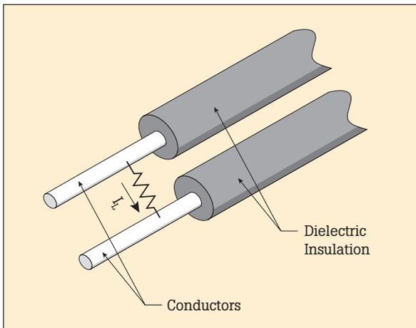
Figure 2. Conductive leakage current ( $I_L$ )
