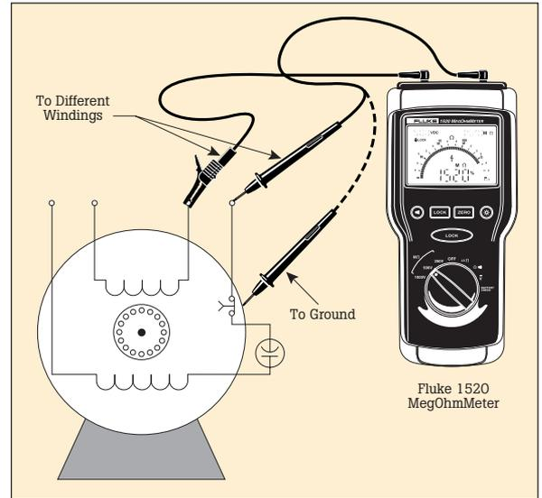
Figure 11. Testing the insulation resistance of a motor
