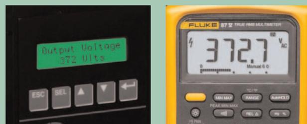
Figure 2. Output voltage reading with low pass filter enabled.
