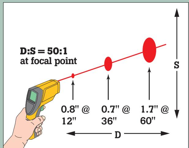
**Figure 2.** Use the Fluke 68 within 8 m (25 ft.) of the intended target. At greater distances, the measured area will be larger (approximately the distance divided by 50).
