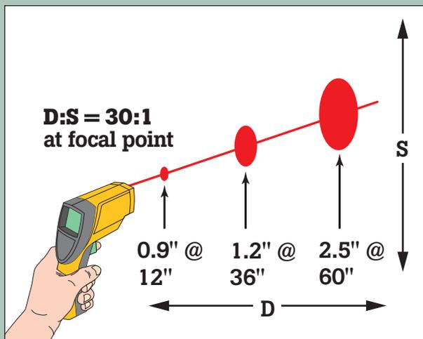
**Figure 1.** Use the Fluke 66 within 5 m (15 ft.) of the intended target. At greater distances, the measured area will be larger (approximately the distance divided by 30).
