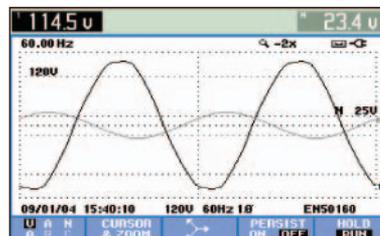
Fig. 2 High neutral waveform
