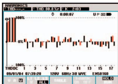
K-factor measures the heating effects of harmonics on transformer loading and losses. K-1 is the baseline for a standard transformer. K-4 would be for times the "normal" heating. K-rated transformer are specifically designed to handle harmonics.
