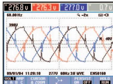
Next, he selected Power & Energy from the menu and compared the kVA calculated by the analyzer to the transformer nameplate's kVA. Sure enough, this transformer was heavily loaded (> 50 %). That meant harmonics were also a concern.
