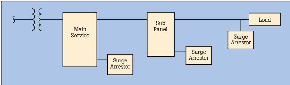
Surge arresters installed at service, panel, load.
