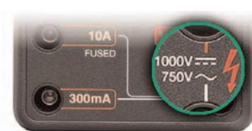
Do not use meters without proper CAT markings on 480 V circuits
