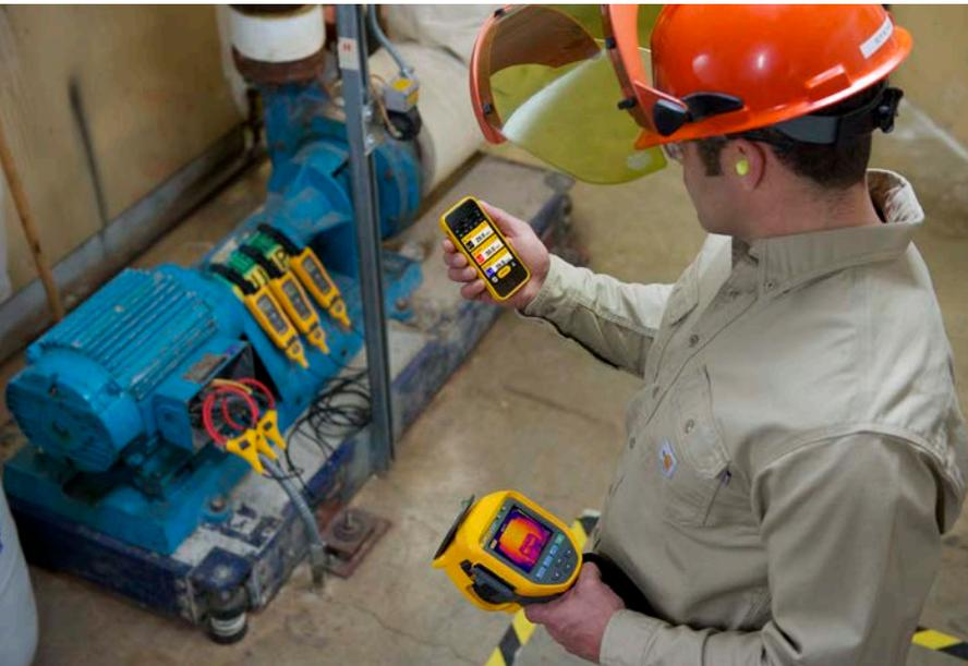
If the temperature or thermal pattern is markedly different from previous readings, you can use other maintenance technologies—vibration analysis, motor circuit analysis, airborne ultrasound, and lubricant analysis—to assess the severity of the problem and the time needed to repair it.
