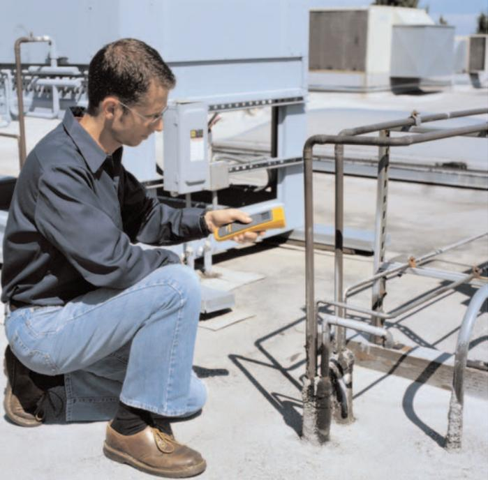
Testing roof-top refrigeration with a Fluke 61 Infrared Thermometer.
