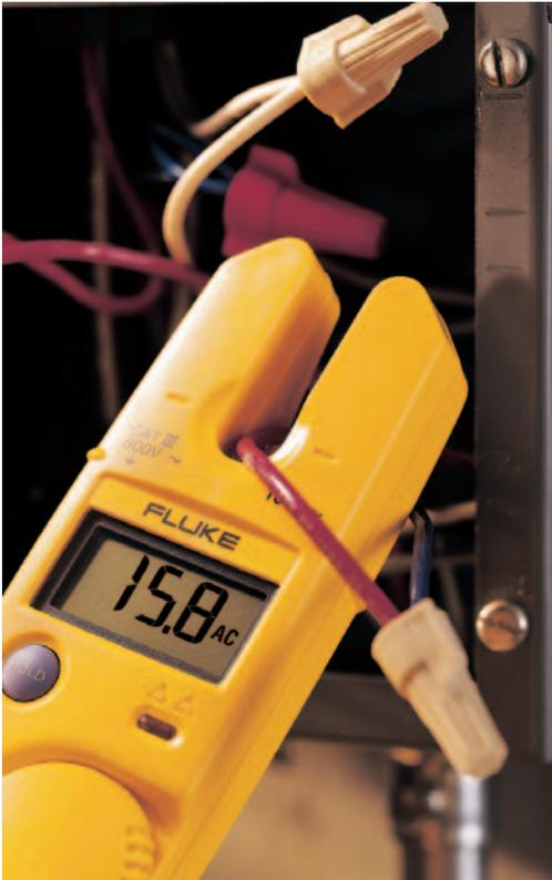
Measuring current with the Fluke T5 Electrical Tester.
