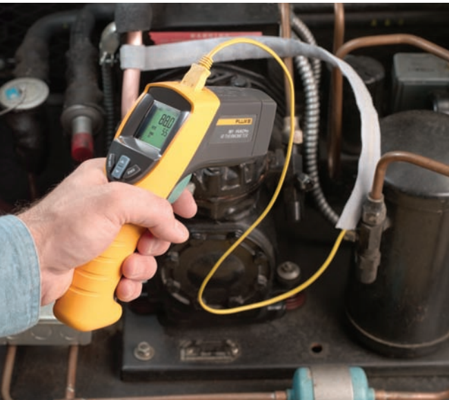
Checking temperature with the Fluke 561 thermometer and Velcro® type K thermocouple.
