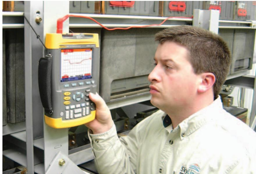
**Measuring tools:** Fluke ScopeMeter® 196C Test Tool
