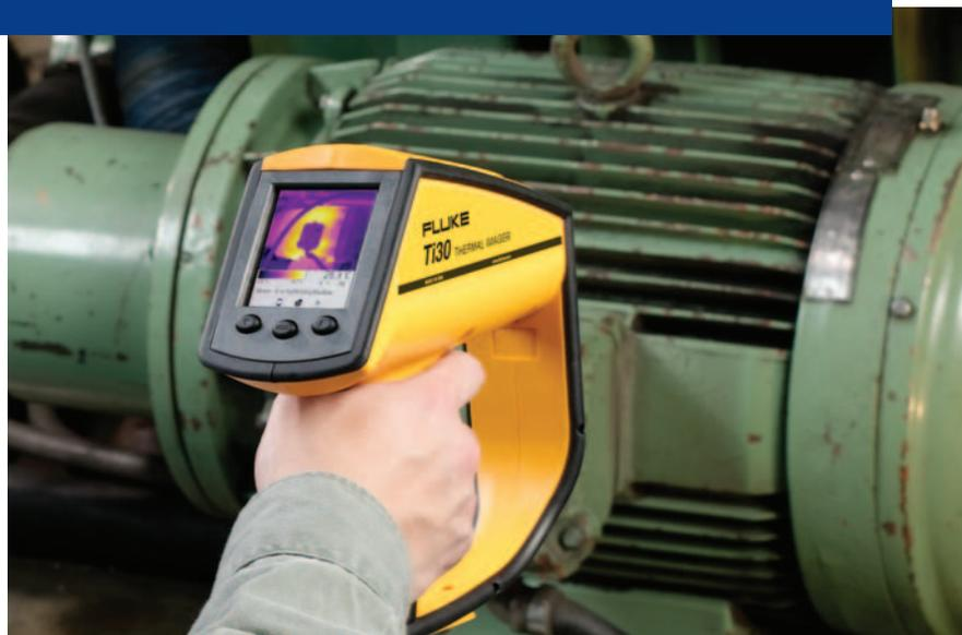
The technology behind the Ti30 is as powerful as the instruments used by specialists, but it makes thermal imaging a point-and-shoot process. It has ample on-board computer power to collect data for a PdM program, and it interfaces with software on a host computer or network, so that maintenance managers can track temperature measurements and compare thermal images over time.
