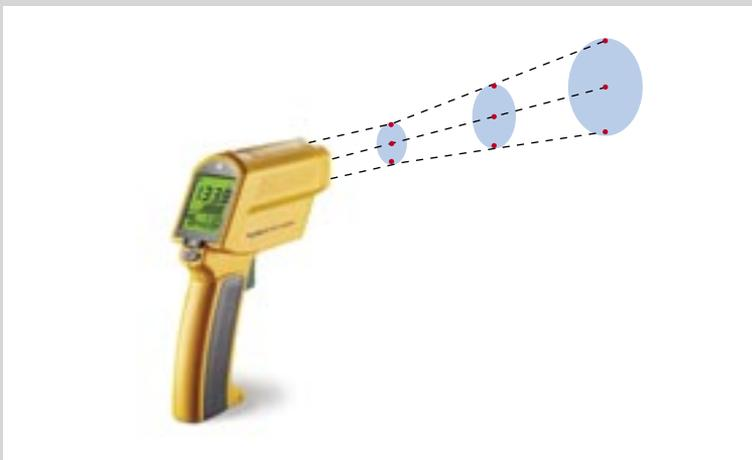
Accurate measurements depend in part on accurately sighting a target. Fluke 570 series thermometers are the only thermometers with a sighting system designed to precisely track the infrared path as seen by the sensors. This enables the advanced coaxial three-dot laser sighting to accurately show both the center and the edges of the spot being measured, regardless of the thermometer's distance from the target.
