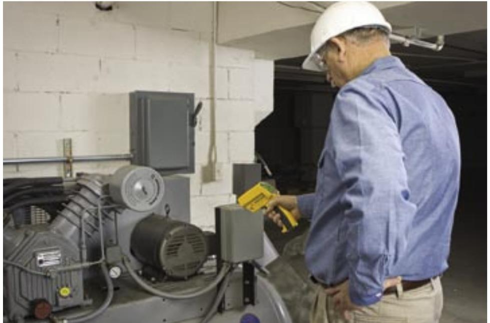
Accurately measure surface temperatures of hot, hard-to-reach, energized or moving objects.
