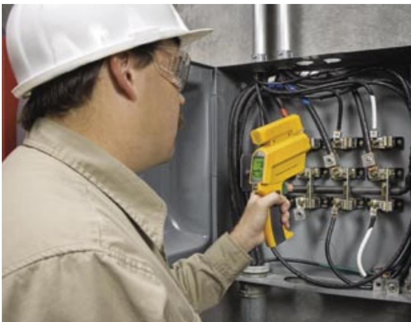
Close focus models and coaxial laser sighting aid small target measurements.
