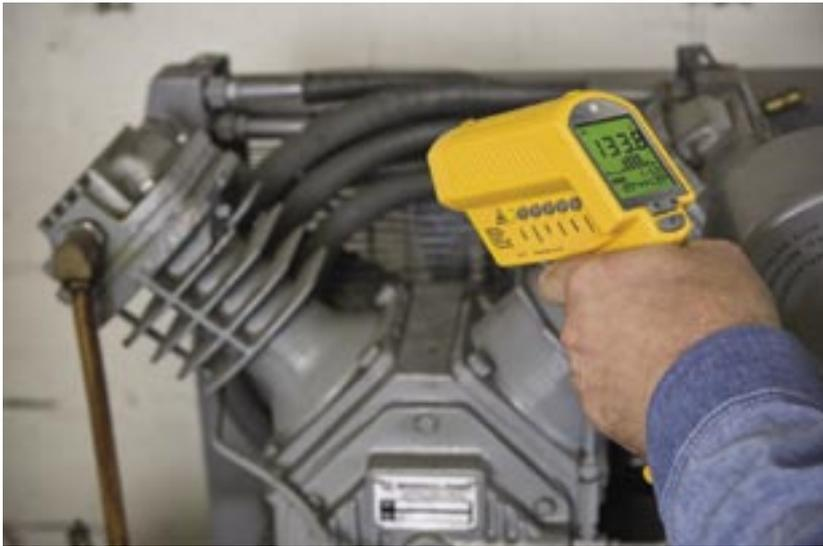
Routinely monitor equipment for temperature changes indicative of possible equipment problems.
