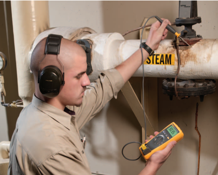
Riko Cus uses the Fluke 179 to check surface temperatures as part of regular monitoring procedures.
