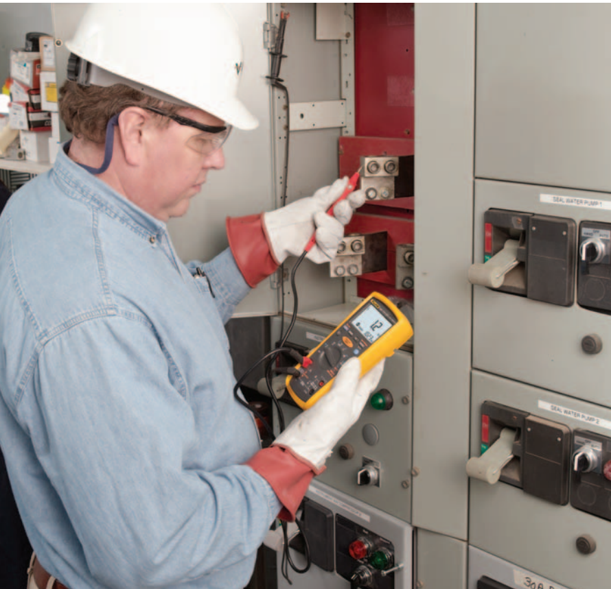
Steve Uhrich of Valley Electric using the Fluke 1587 Insulation Multimeter.
