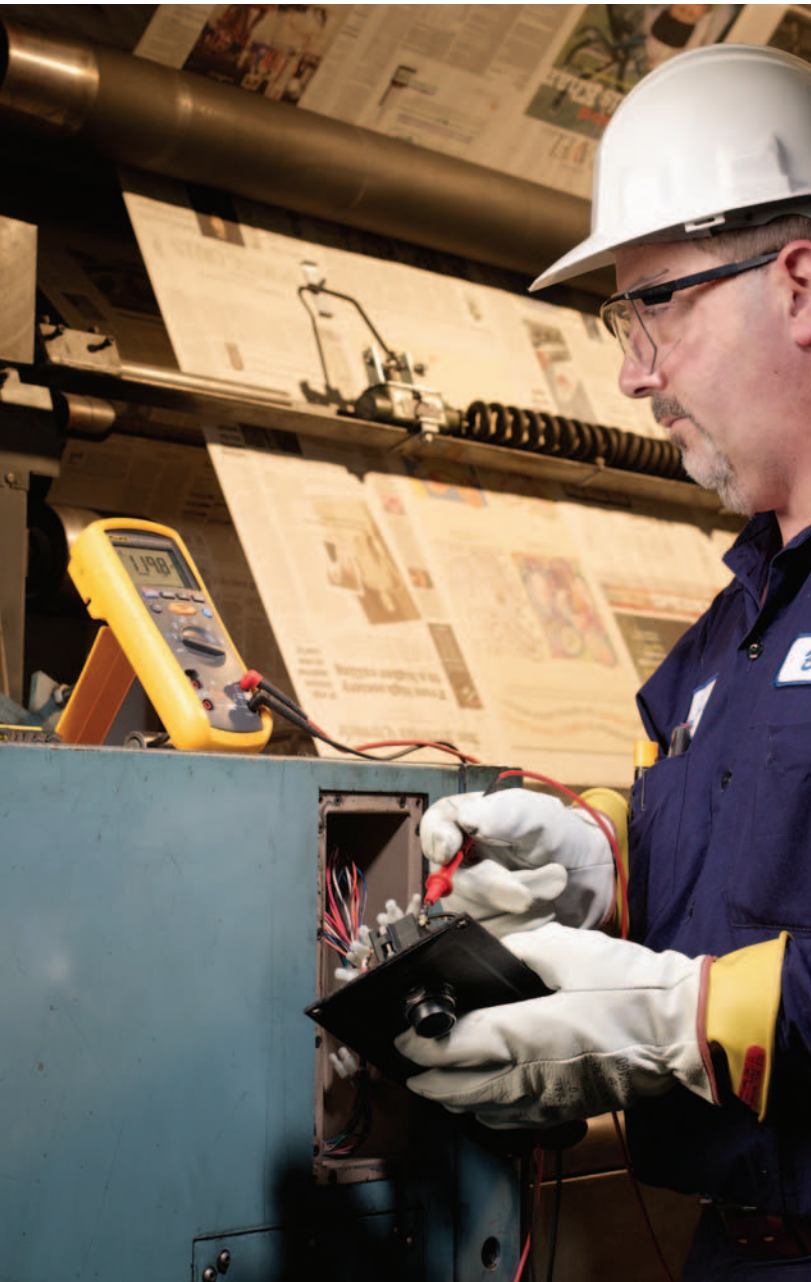
Bill Weindorf using the Fluke 1587 Insulation Multimeter.
