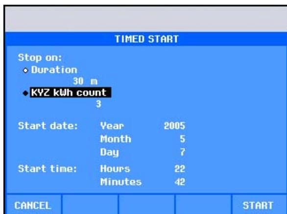
**Figure 6.** Setting the number of pulses to count.
