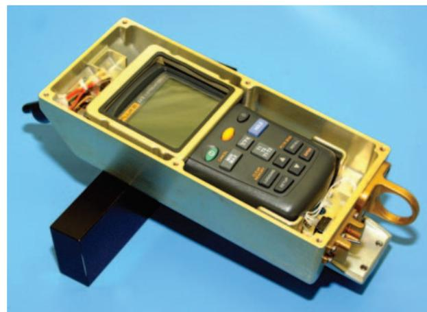
NASA engineers disassembled 10 Fluke 54-2 thermometers to create their custom space-models. In the process, they investigated every safety aspect imaginable, especially shatter-proof impact resistance and extreme temperature tolerance.
