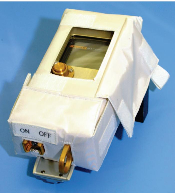
The Fluke 54-2 in its NASA suit of aluminum, mylar and fiberglass. Engineers reduced the controls to just one button.
