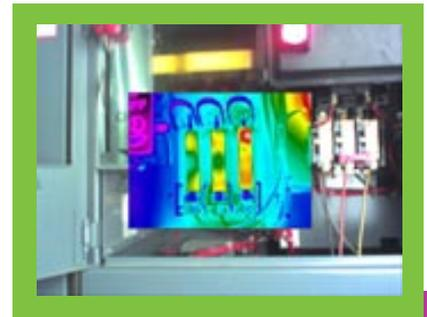
Fluke thermal imagers now include IR-Fusion<sup>®</sup>\*, a technology that fuses a visual, or visible light, image with an infrared image for better identification, analysis and image management. The dual images are accurately aligned at any distance heightening details so problems are easier to spot.
