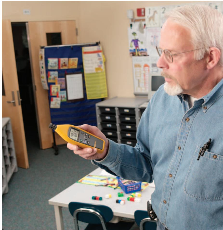
Measuring ambient temperature and relative humidity to evaluate air comfort.
