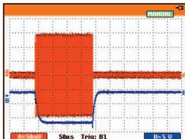
Figure 4: At lower timebase setting, the 'glitch detect' function builds a solid envelope of a high frequency burst (Fluke 199C).
