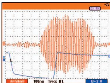
Figure 5: A short duration burst is captured, but the envelope is more difficult to identify (Fluke 199C).
