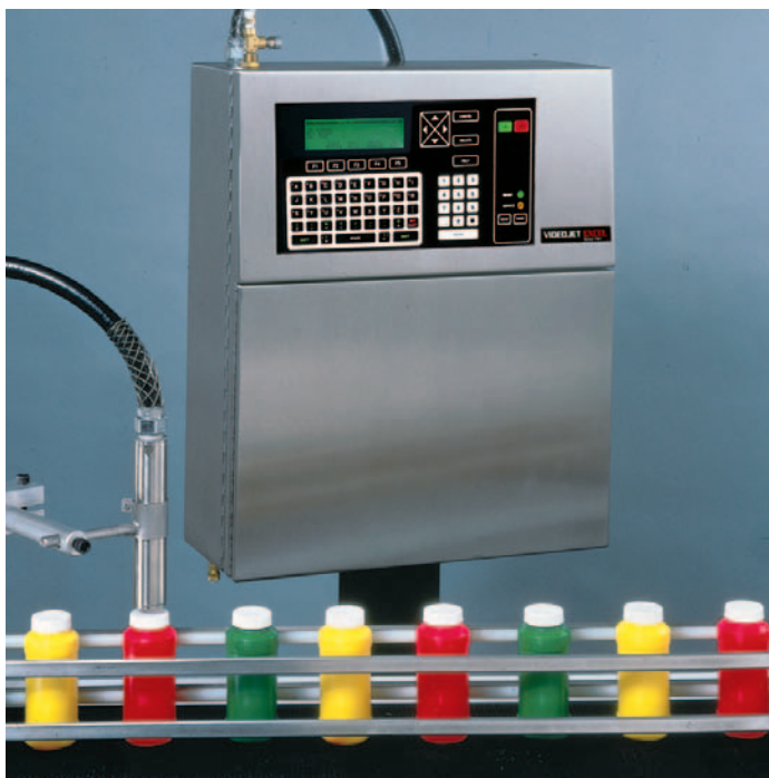
Figure 5: VideoJET Excel printer in a production line.
