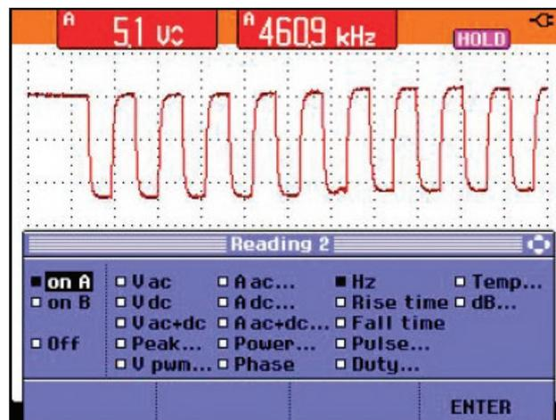
**Figure 1:** Peak-to-Peak voltage and frequency are measured simultaneously.
