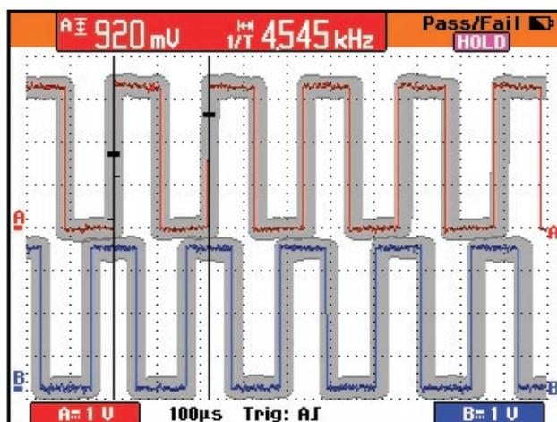
Figure 2: ScopeMeter screen shots showing envelopes created over two encoder signals.
