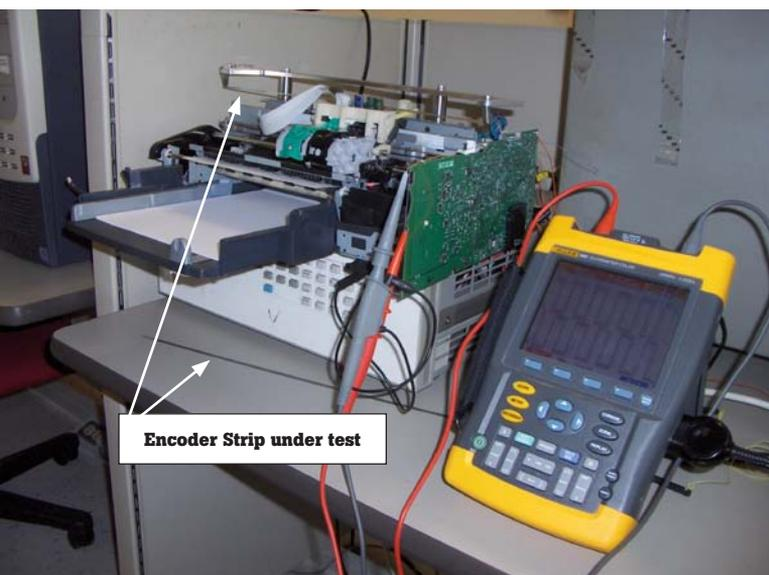
Figure 3: Carriage Encoder Test Fixture.
