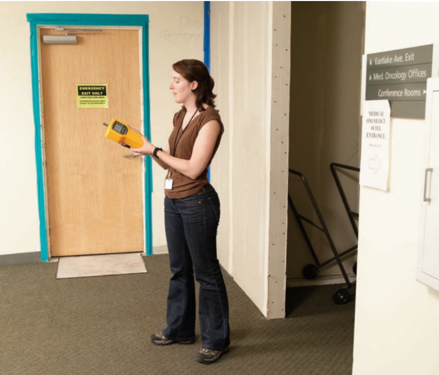
Collecting airborne particle counts in the occupied space using the Fluke 983.
