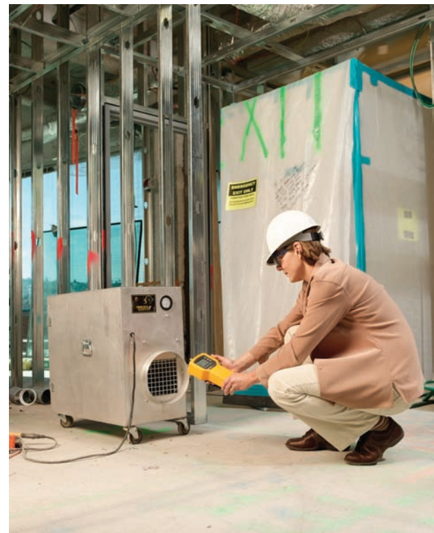
Checking particle counts in an air scrubber's supply air using the Fluke 983 Particle Counter.
