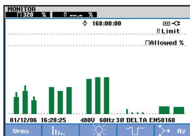
System monitor summary shows pass/fail results for average voltage, harmonics, flicker, dips, unbalance and frequency. In this case all parameters were in tolerance.
