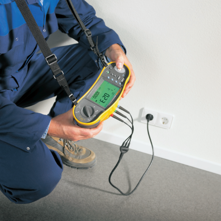
Electrician in Europe using the Fluke 1653 to test a receptacle.
